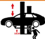
Stop and check lift arm locks and stability of vehicle after short raising, then to desired height.
